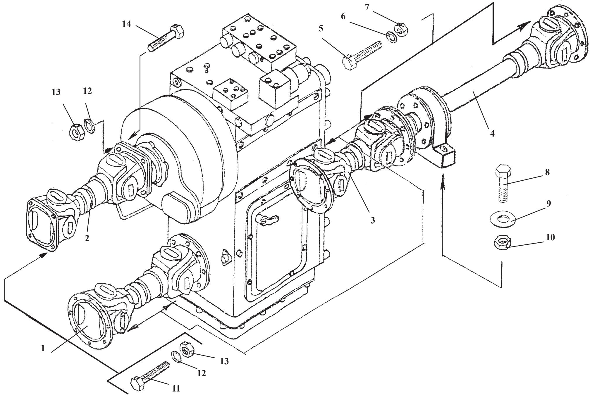
Propeller shafts Setup
